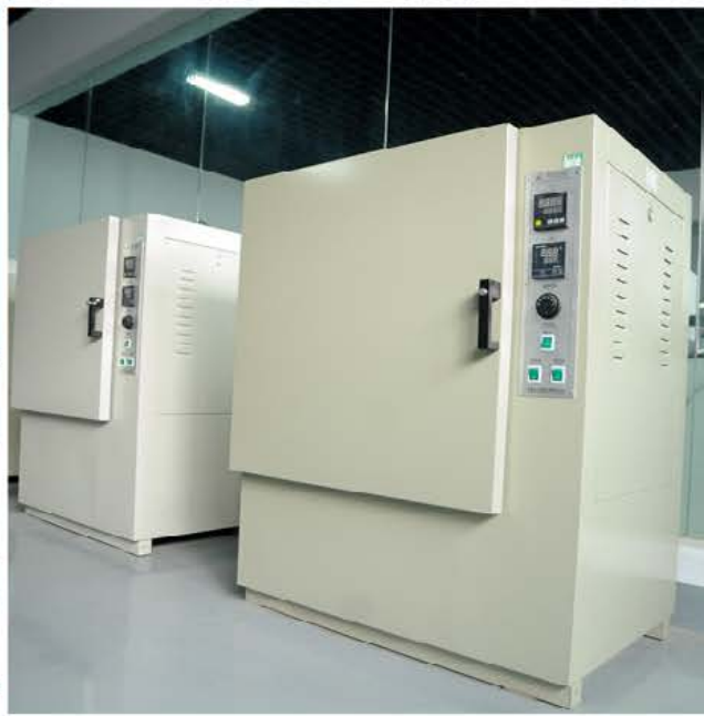
◀ Thermal stability testing machine (left) Gel content determination device (right)
