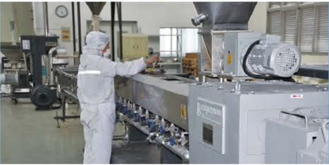
Extruding machine Si- XLPE( Silane cross-linked polyethylene insulation compound )
